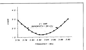
fig. 5. VSWR plot between 3.76 and 3.90 MHz of the 75-meter system.
