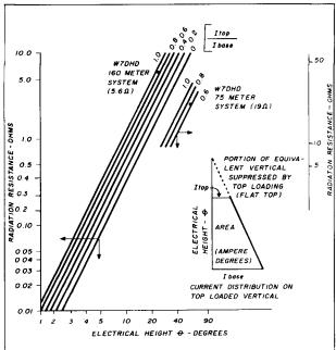
fig. 4. Radiation resistance versus angular aperture (electrical height),  $\theta$ , for top-loaded vertical antennas.<sup>2</sup>
