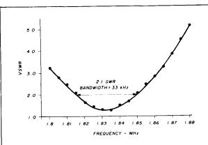
fig. 4. VSWR plot between 1.800 and 1.880 MHz of the 160-meter system.
