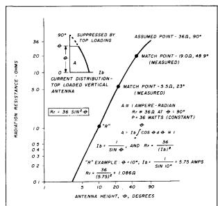
fig. 5. Radiation resistance of top-loaded vertical antennas from 3 to 90 degrees. Theoretically derived and modified to fit measured resistances ( $\Delta r$  less than 1 ohm at  $\theta=50$  degrees).
