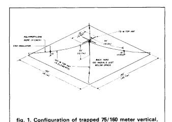
The system is resilient enough so that continued vibration certainly would not have damaged the structure, but it does stranger things: it unscrews nuts, bolts, and machine screws, and it causes fatigue in electrical connections. The fastening points for the guys on the mast are steel devices designed for connecting 2-inch fence posts together. All guys are broken up into sections approximately 10 feet (3 meters) long, insulated by TV-mast-type "egg" strain insulators.
