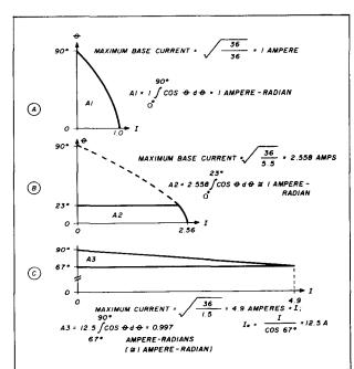
fig. 1. Current distributions for three referenced antennas, each over perfect ground, and 36 watts input to antenna terminals. All to scale, so areas are directly comparable. (A) Current distribution of  $\lambda/4$  vertical (reference antenna) against a perfect ground, (B) Current distribution of  $\lambda/16$  (23 degree) top-loaded vertical against perfect ground, (C) Current distribution of  $\lambda/16$  (23 degree) base-loaded vertical against perfect ground.
