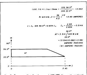
fig. 3. Current distribution on  $\lambda/16$  (23 degree) vertical antenna with equal top- and base-loading, over perfect ground, no coil loss. (Same scale as figs. 1 and 2.)
